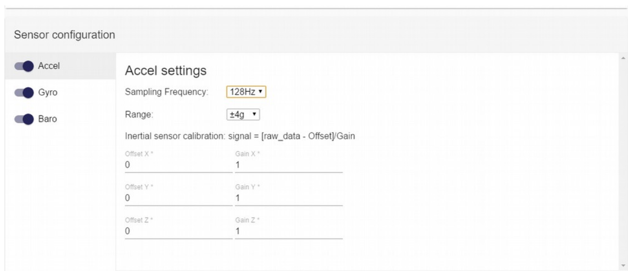
Illustration 4: Sensor configuration possibilities: You can activate/inactivate each sensor and set the sampling frequency. For accelerometer and gyroscope you can in addition set the maximal range and the calibration values
